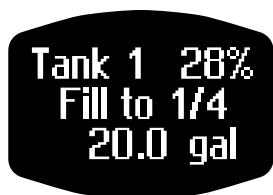
Figure 1-53: Setting Tank Calibration Points for 25-100%
